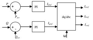
*Figure 3:* Block diagram of PQ inverter control system *b) VF control mode*
