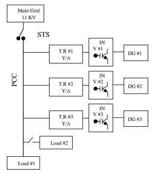
Figure 6: Single line diagram of the proposed system.
