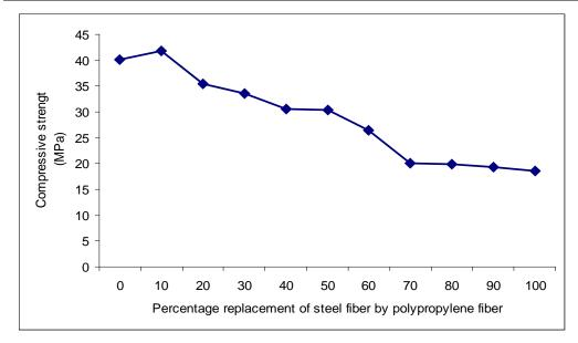
*Figure 1 :* variation of Compressive strength of slurry infiltrated fibrous fibrocement with partial replace mentof steel fiber by polypropylene fiber.
