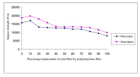
*Figure 3*: Variation of impact strength of slurry infiltrated fibrous ferrocement with partial replaceme of steel fiber by polypropylene fiber.
