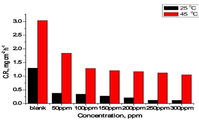
Figure 4 : Corrosion rates of various concentrations of expired Cidamex on aluminum in 1 M HCl at 25 and 45°C
