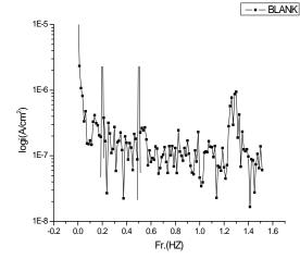
Figure 10: Intermodulation spectra recorded for carbon steel electrode in 1M HCI solutions in the absence and presence 300 ppm of expired Cidamex
