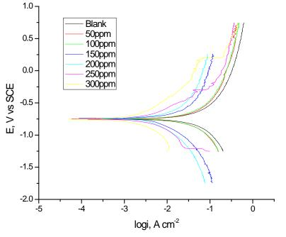
Figure 8 : Anodic and cathodic Tafel polarization curves for aluminum in the absence and presence of various concentrations of Cidamex
