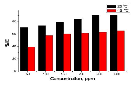
Figure 5: The variation of inhibition efficiency with expired Cidamex concentration of aluminum in 1 M HCl solution Table 1 : Data from weight loss of Al in 1 M HCl for various concentration of expired Cidamex after 1.5 h at 298 and 318 K
