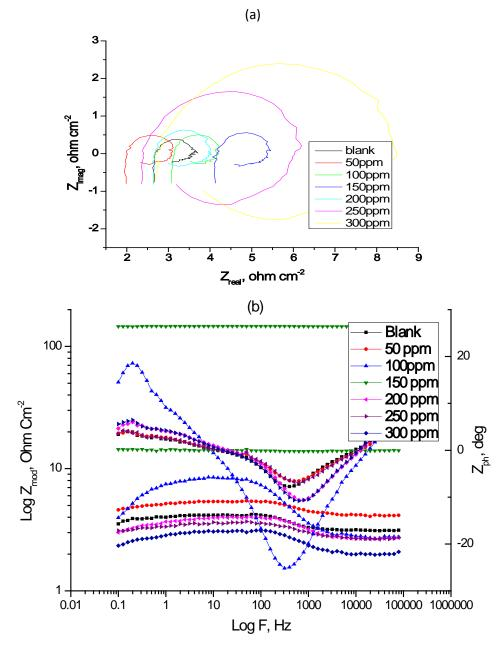
*Figure 9 a, b :* EIS results for aluminum in the form of Nyquist Bode plots for expired Cidamex at different concentrations and at 25°C
