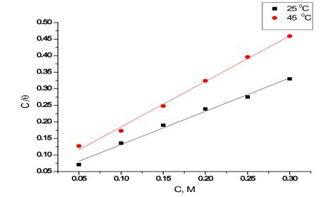
*Figure 6 :* Langmuir adsorption isotherm for expired Cidamex adsorption on aluminum in 1 M HCl at two different temperatures after 1.5h immersion
