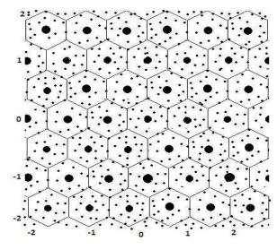
*Fig. 3:* LTE-A cellular network using regular hexagonal cell.
