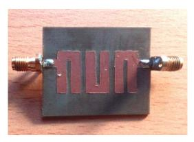
Fig 4.2: Fabricated 3.5 GHz Filter
