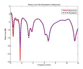
Fig.3.4: Simulated and Measured Return Loss Plot
