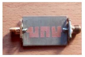
Fig 4.4: Fabricated 7.5 GHz Filter
