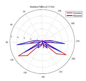
Fig 5.7: Radiation Pattern at 7.5 GHz
