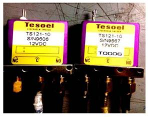
Fig 4.7: Teseol SPDT switches
