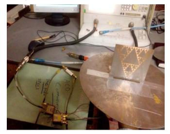
Fig.5.3: The Sierpinski Monopole Antenna along with Filters and Switches
