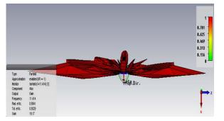
Fig. 3.10: 3D Radiation Pattern at 3.5 GHz
