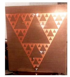
Fig.3.3: Fabricated Sierpinski Monopole Gasket
