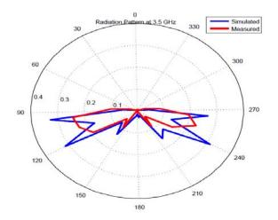
Fig.5.6: Radiation Pattern at 3.5 GHz
