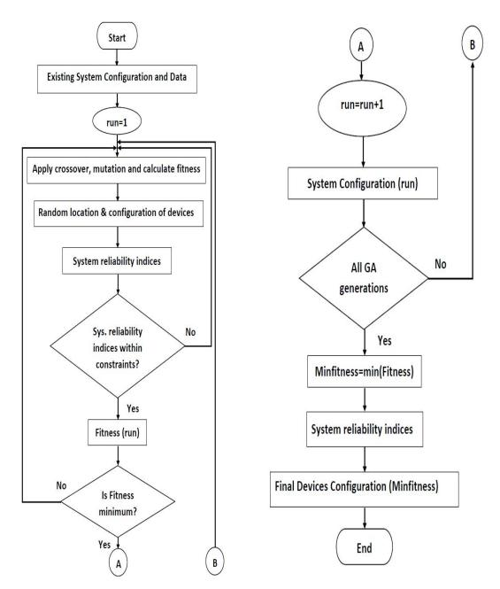
Fig. 2: Automation, reclosing and switching flow chart for genetic algorithm optimization
