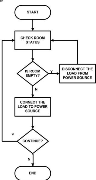
Figure 4 shows the program flow chart for the automated switch. The primary aim of the program was to determine wither the room was vacant or not. And
