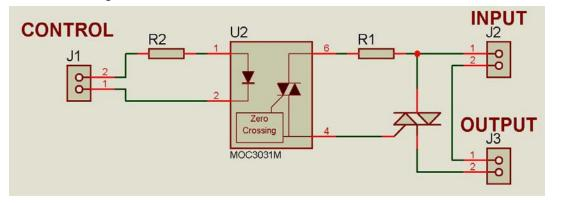
Figure 3: Solid State Relay (SSR)
