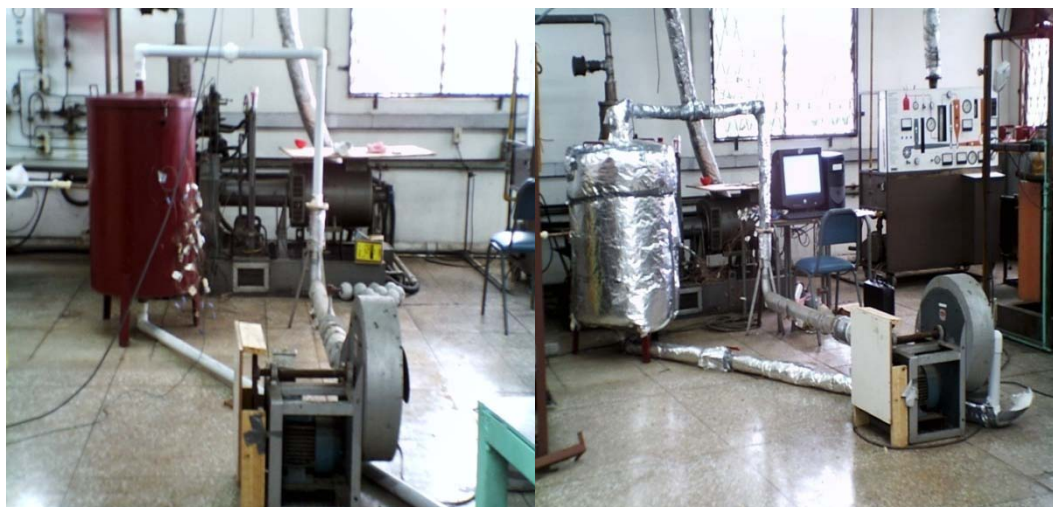
Figure 3.0 : A photograph of simultaneous charging and discharging packed bed energy storage system components before and after insulation
