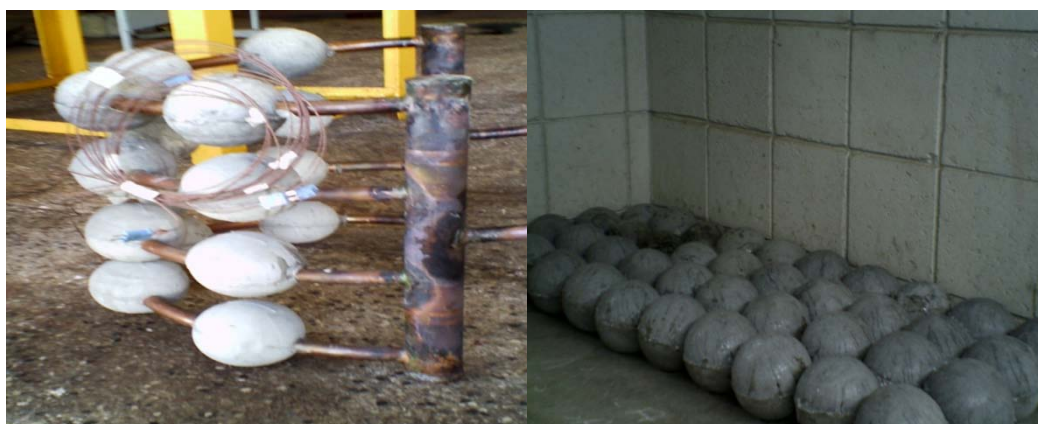
Figure 4.0 : A photograph of spherical shaped concretes and those imbedded with copper tube
