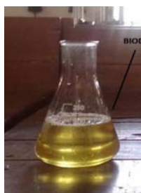
Fig 5 (c) : Extracted crude biodiesel
