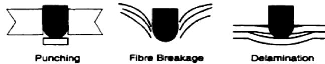
Figure 2 : Damage mechanisms occurred in composite materials under ballistic impact[9]
