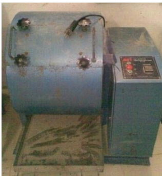
Figure 10 : Test Cantabro Machine
