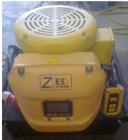
Figure 2 : The loading device (model Enerpac-ZE5)
