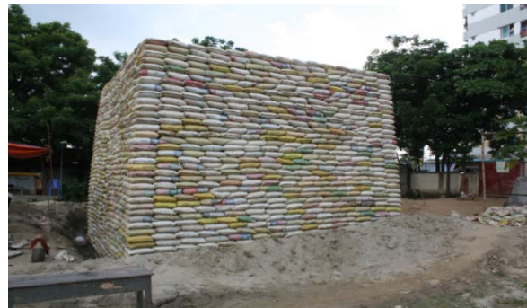
Figure 2: Sand Bag used for loading the pile
