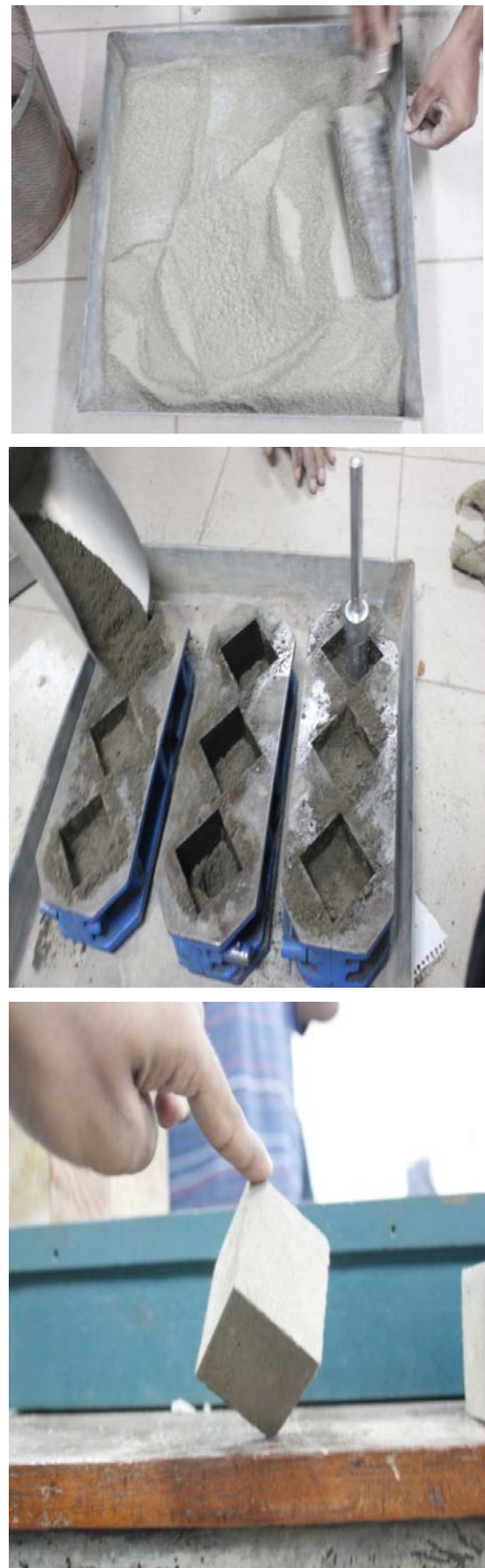
Fig. 2: Final Sample of Soil-Cement Block
