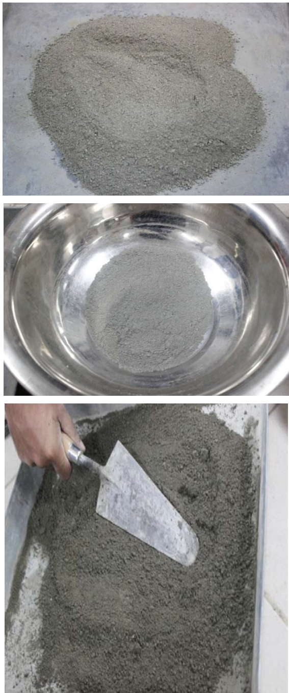
Fig. 1: Soil Cement Mixing and Moulding
