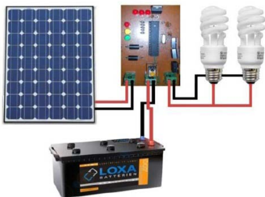
Figure 1C : Basic image of controller and battery wiring [18]
