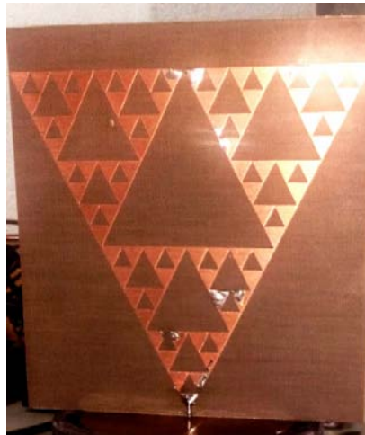
Fig.3.3: Fabricated Sierpinski Monopole Gasket
