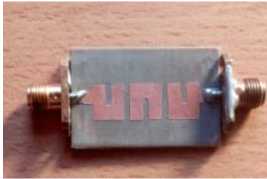
Fig 4.4: Fabricated 7.5 GHz Filter
