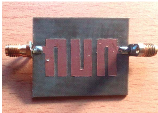
Fig 4.2: Fabricated 3.5 GHz Filter
