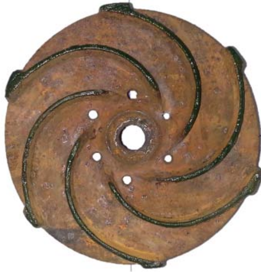
Figure 1: Centrifugal impeller with backward blades
