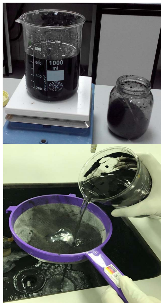
Figure 5: Manganese oxide washing
