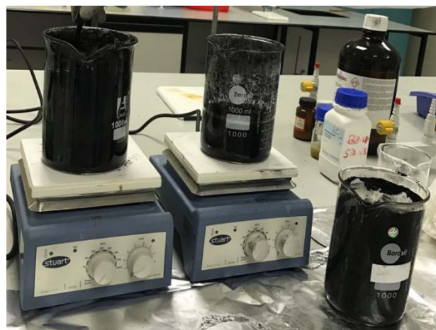
Figure 7: Manganese dioxide paste heated
