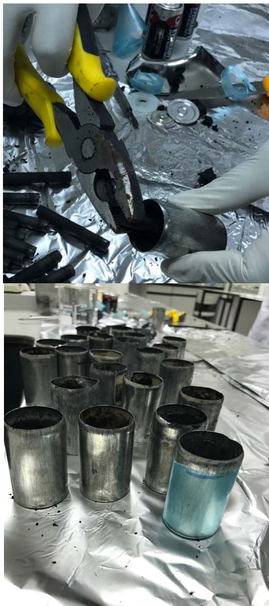
Figure 4: Battery graphite cathode removal
