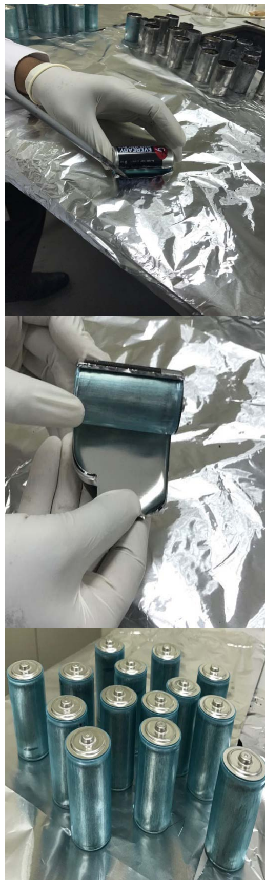
Figure 3: Battery outer cover removal
