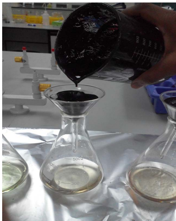
Figure 10: Manganese sulphate solution filtered
