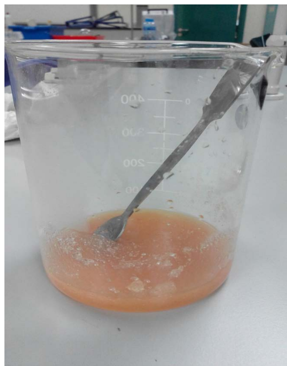
Figure 12: Manganese sulphate crystals
