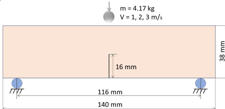
Figure 2: Impact experimental setup of PMMA beam
