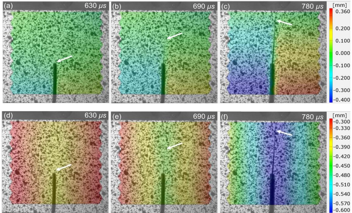
**Figure 5:** Crack initiation and propagation at different time steps, with the corresponding displacement fields (displacements in x direction: (a), (b), and (c); displacements in y direction (d), (e), and (f)) in the PMMA beam after the impact at the velocity of 1 m/s. (The crack tips are marked with the white arrows)
