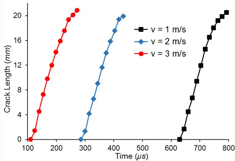
Figure 8: Crack initiation and propagation length history in PMMA beams subjected to impact with different impact velocities
