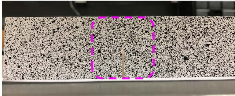
Figure 3: PMMA beam surface preparation for DIC
