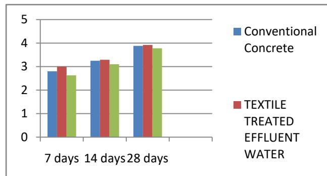
c) *Flexural Strength Concrete in Prism*
