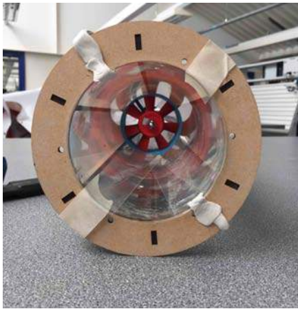
Figure 6: Image shows the Outlet view of the wind tunnel
