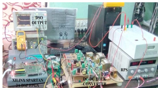
Fig. 24: Experimental setup for the Modified DPI enabled DPWM based DC-DC buck converter using FPGA
