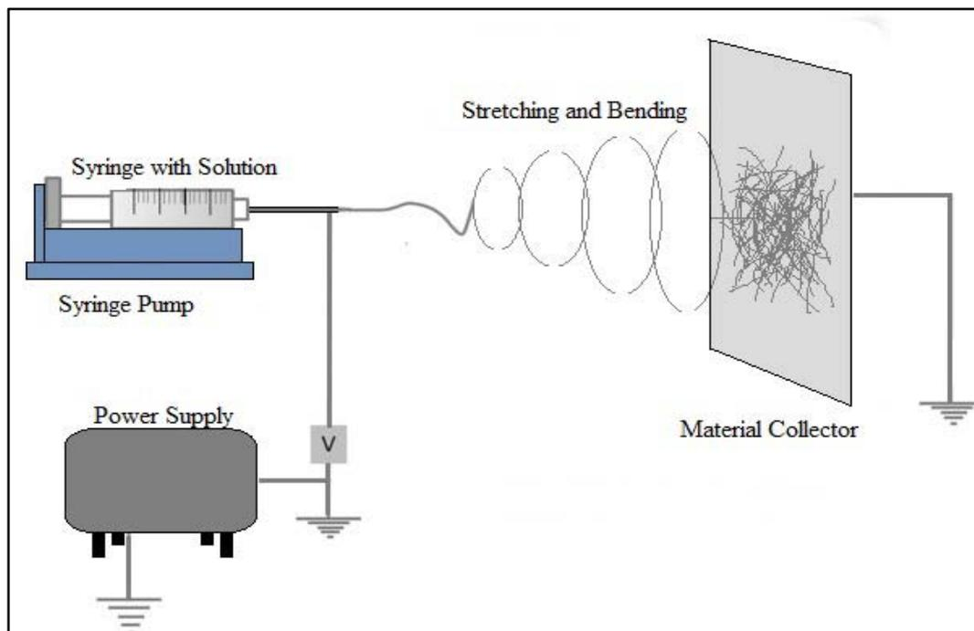
Fig.1: The Electrospinning process schematic
