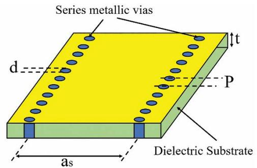
**Fig. 1:** Layout of Basic SIW structure realized on a dielectric substrate ( $a_s$ =effective width of SIW section,  $p$ =center to center gap between vias ‘pitch’,  $d$ =diameter of metallic vias and  $t$ =thickness of dielectric material).
