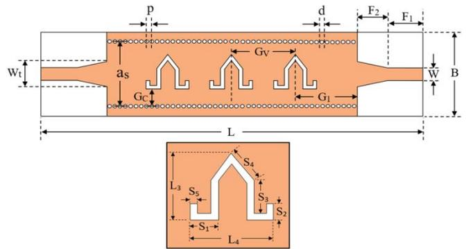
Fig. 4: 180° FMSIW bandpass filter with EBG realized on a dielectric substrate
