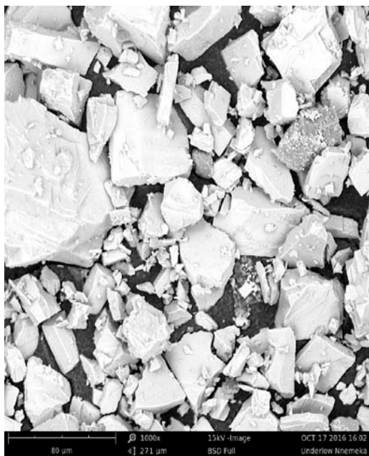
Fig. 4: SEM Microstructure of the Jigging underflow
