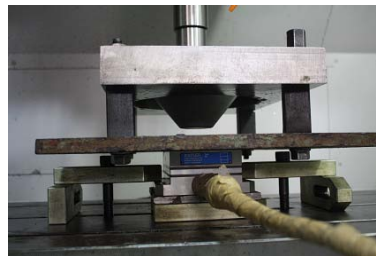
Fig. 6: Force measurement setup in SPISF
