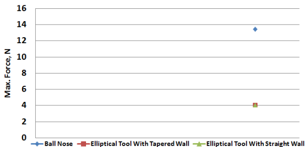
Fig.10: Comparison of maximum force for different tool geometries in case of tool diameter 7 mm and wall angle 50°
