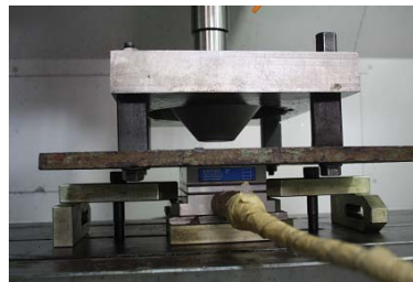
Fig. 6: Force measurement setup in SPISF
