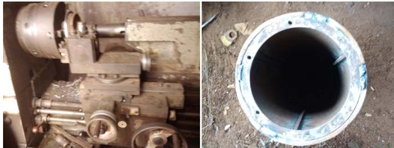
Fig. 5: Marking the rings using the dividing head; machined rings welded to the pipe
