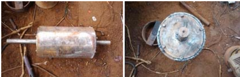
Fig. 8: Flanges fastened to the pipe using M8 bolts
