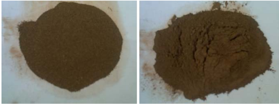
Fig. 17: Limestone product (a) after grinding (b) after sieving
