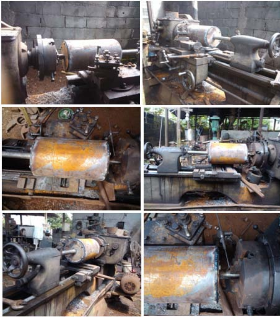
Fig. 9: Different views on how the pipe and flange assembly were mounted on the lathe machine and the scribing of the mounted assembly
