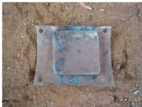
Fig. 13: Square cut out part welded to a curved plate to serve as feed hole cover
