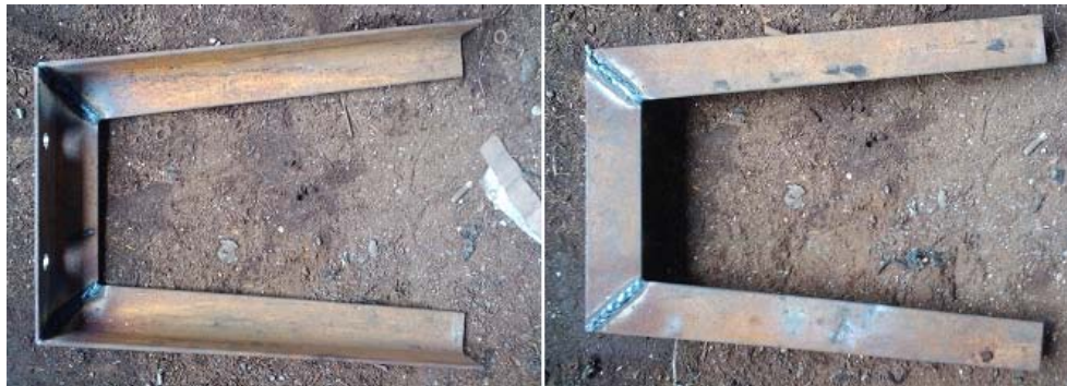
Fig.10: Different views of the welded legs of the stand
