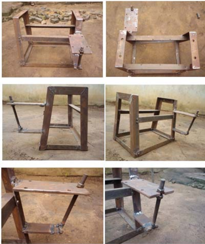
Fig. 14: The different views of the assembled stand and a clearer view of the motor seating
