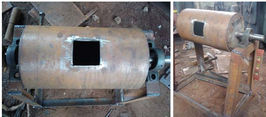
Fig. 12: Feed and discharge hole cut on the vessel
