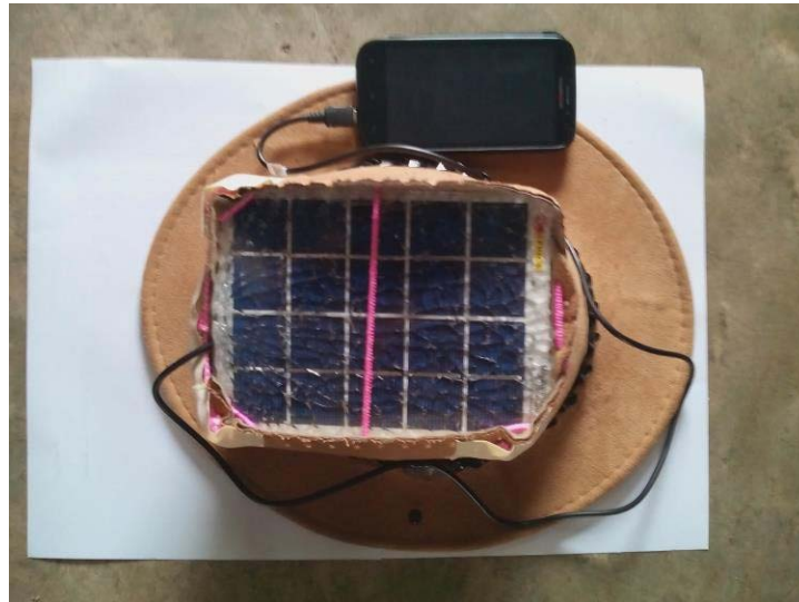
Figure 3.2: Direct charging of battery of a mobile phone
