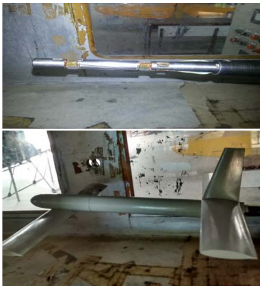
Fig. 16: Wind Tunnel Balance and Scaled Model
