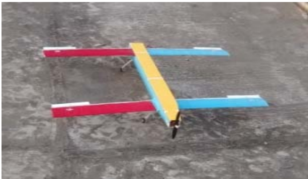
Fig. 21: Prototype made of Composite material and multigrain
