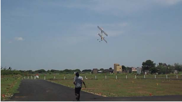
Fig. 20: Flight test of Tandem wing aircraft
