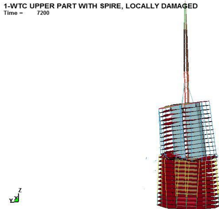
Fig. 8 As a result of wall damage the upper part of the building tilts and begins to fall. This motion can't be stopped
