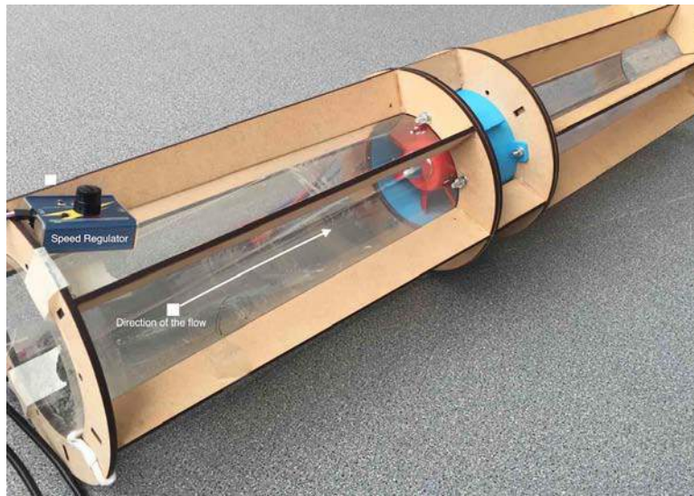
Figure 4: Image shows a Wind tunnel includes impeller and fan case
