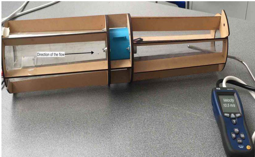
Figure 7: Image shows Manometer is connected without fixing the ends, which cause vibrations. The averaged outlet velocity, mass flow and thrust measured using the manometer are listed in Table 2.
