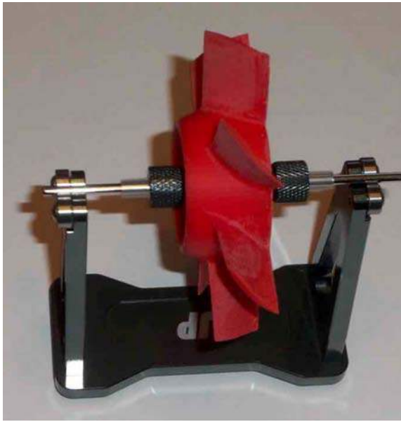
Figure 2: ABS impeller produced by 3 D printing device fixed by alignment shaft
