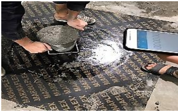
Fig. 1(a): Slump flow T50 test
