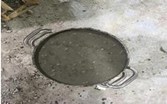
Fig. (1) c: Bleeding test
