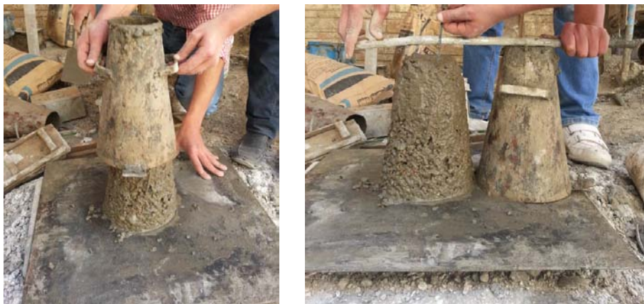
Figure 4: The slump test
