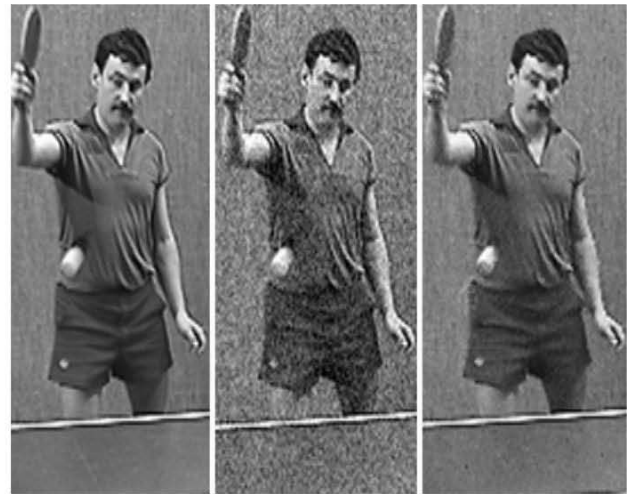
Fig. 5: Denoising of video “Tennis” corrupted with noise \sigma = 20 using ATA method, frame 300; from left to right: original, noisy, denoised.
