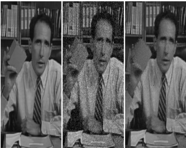
Fig. 4: Denoising of video “Salesman” corrupted with noise \sigma = 20 using ATA method, frame 100; from left to right: original, noisy, denoised.
