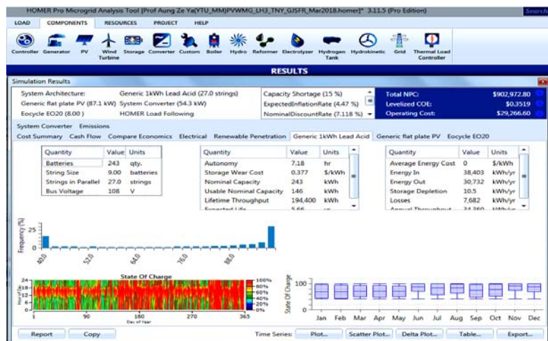
Fig. 27: Simulative Results: Storage Battery System of Proposed Zero-Emission, PV-Wind-Battery Hybrid
