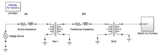
Figure 4: Single Phase Test circuit of EAF
