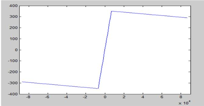
Figure 5: VI-characteristics of model1 in static state
