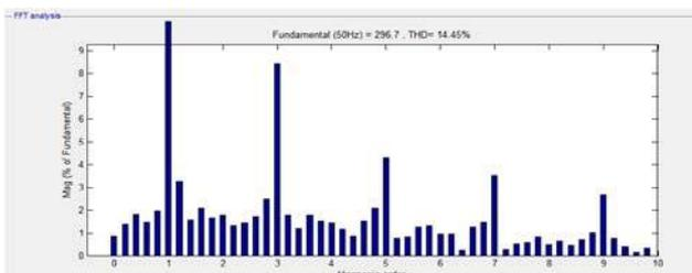
Figure 27: Harmonic spectrum of an arc furnace current during refining
