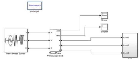
Figure 23: three phases Test circuit of EAF connected supply system.
