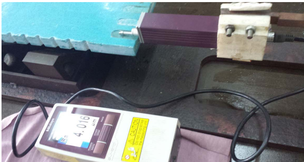
Fig. 5: Experimental setup of measuring surface roughness
