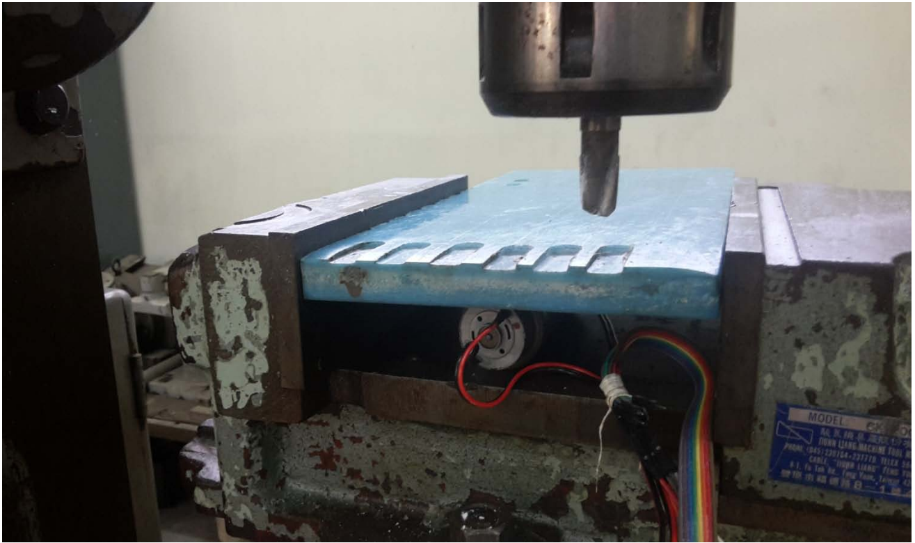
Fig. 1: Vibration device attached to the work piece
