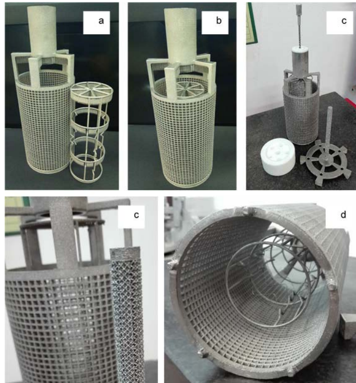
Fig. 6: a - as-built parts of a system with support structures; b - the combined components; c - resolution of lattice structures of an electrode; d - inside the system: the inner dispenser for samples.
