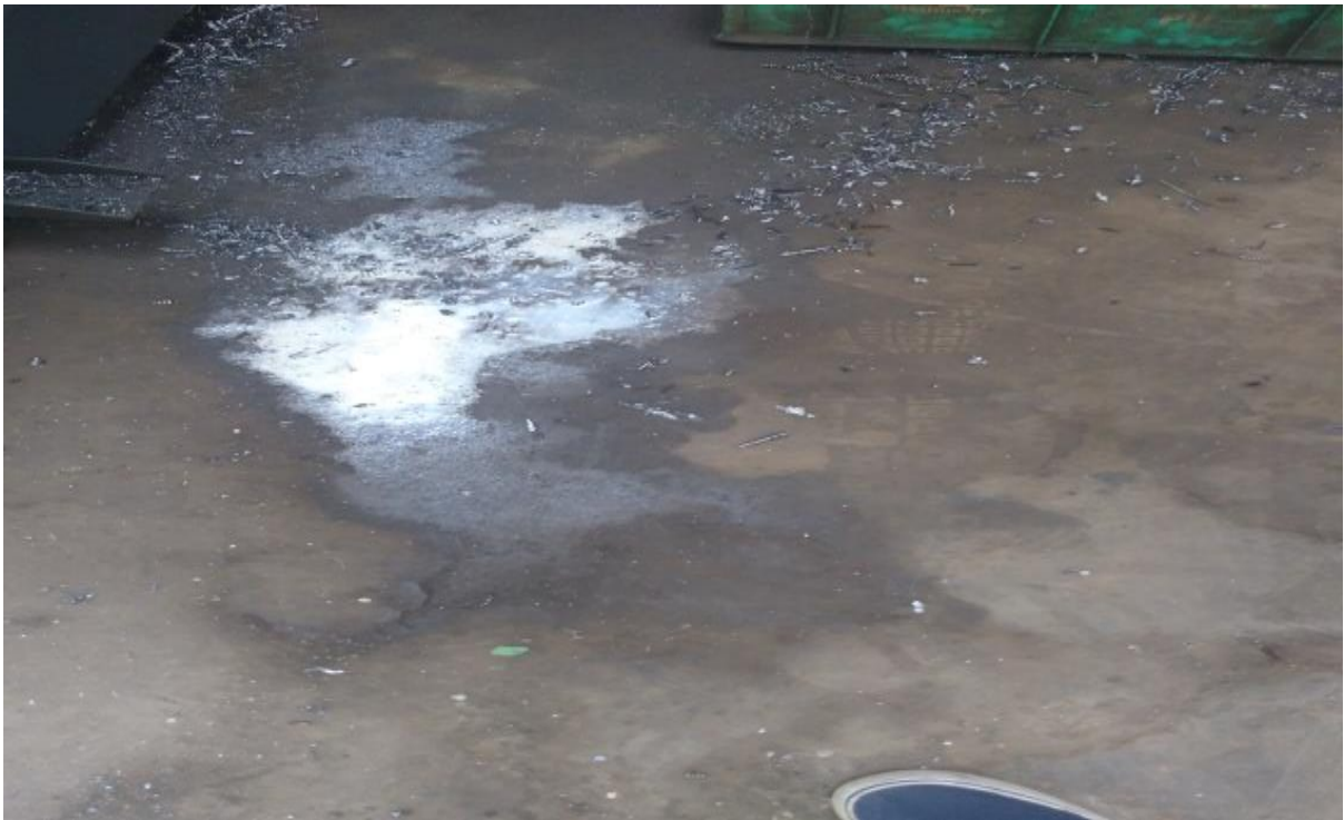
Coolant overflow from the tank is spilled on the ground without any provision to clean it.
