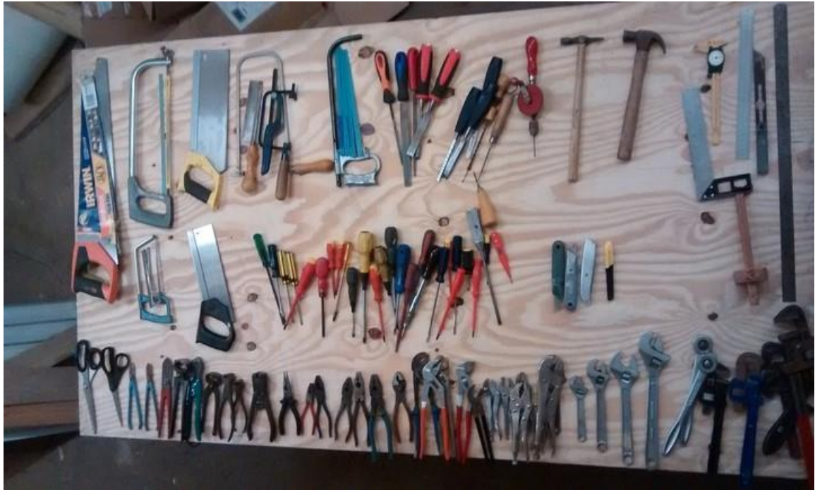
Fig.1.5: Arranged all tools by poke yoke concept
