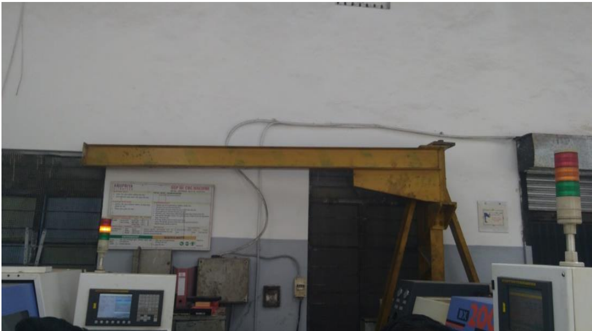
Before - Crane used to load chuck for bell housing is still kept in between CNC machines even after its use is over.
