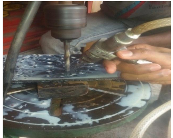
(a) MQL set up (b) Operation performing on MQL
