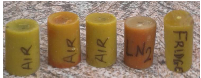
Figure 7: Beeswax samples cooled in various media; air, liquid nitrogen, and refrigerator.
