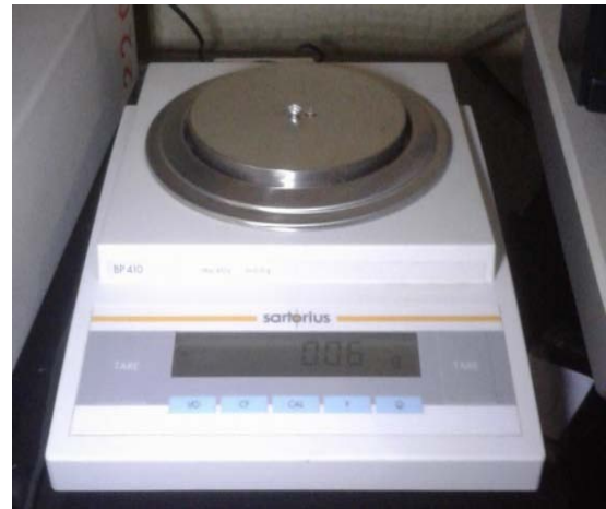
Figure 3: Weighing of the sample with hermetic aluminum sample pan with the lid on Sartorius BP410 digital laboratory balance
