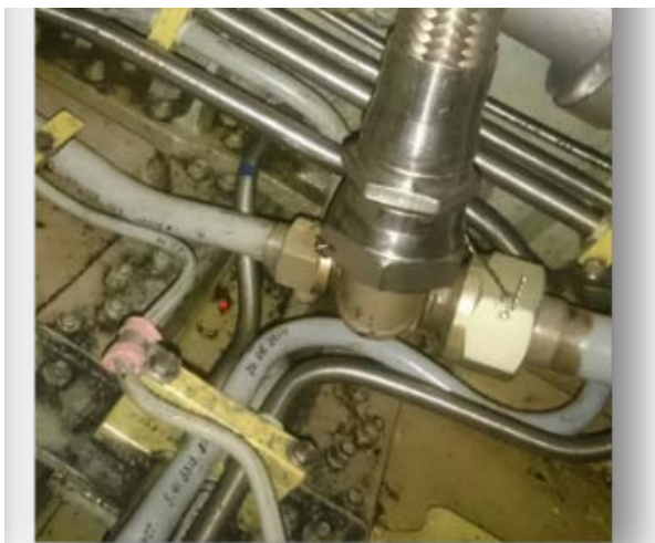
Figure 4: Routing (Zone 1) of a Hydraulic Pipeline and support clamping
