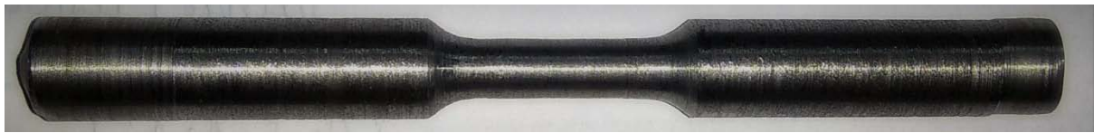
Fig. 2(a): ASTM-E8 EN36C steel Specimen before the tensile test.
