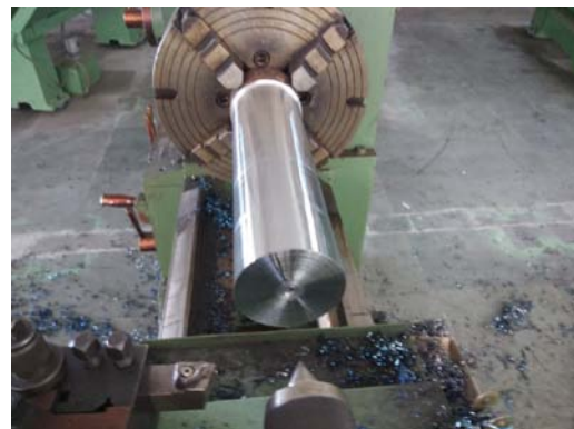
(b). EN36C Steel after machining.
