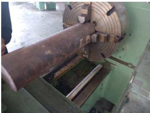
Fig. 1: (a). EN36C Steel mounted on the lathe.
