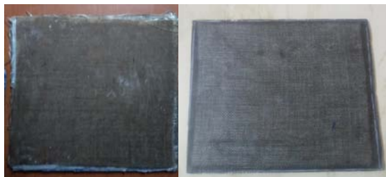
Figure 6: Glass fiber-basalt and glass fiber-jute
