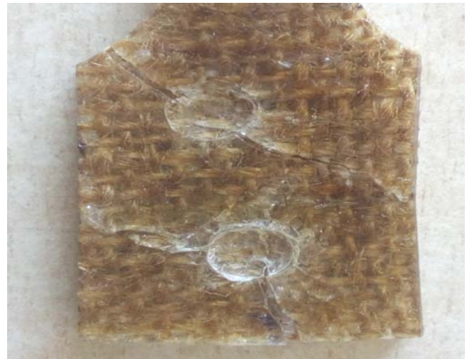
Figure 8: Hardness test in composite material
