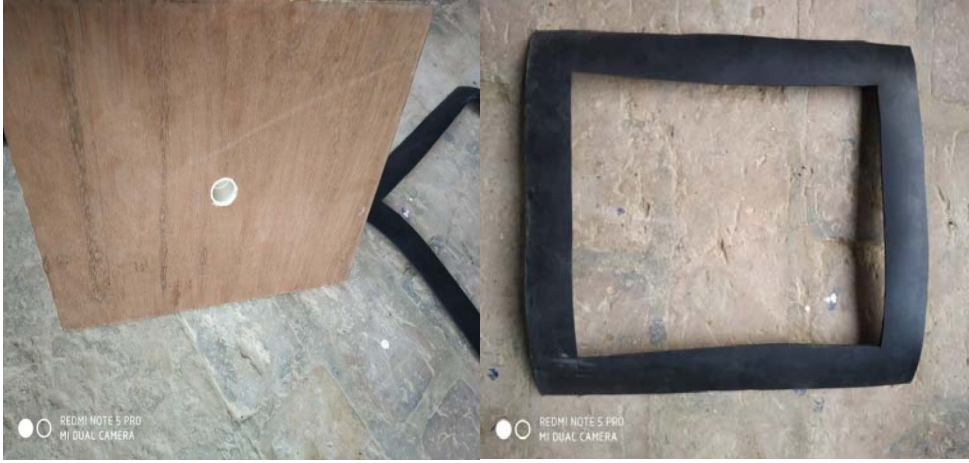
Fig. 2.1: Front view of suction pad while looking from face and the rubber used in the suction pad.
