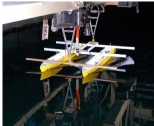
Figure 8: Towing Tank Experiment of Ship Resistance, [3]
