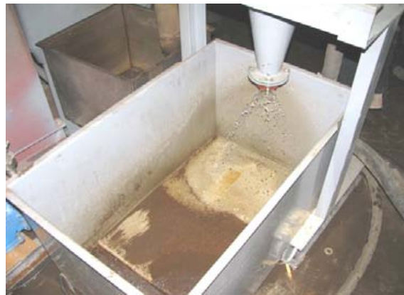
Figure 11: Recycled Water in a Tank after Cleaning in the Filtration System
