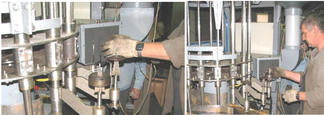
Figure 9: Loading of Contaminated Parts for Cleaning and Unloading the Cleaned Parts.
