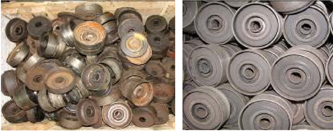
Figure 13: Pump Parts in the Plant Before and After Cleaning
