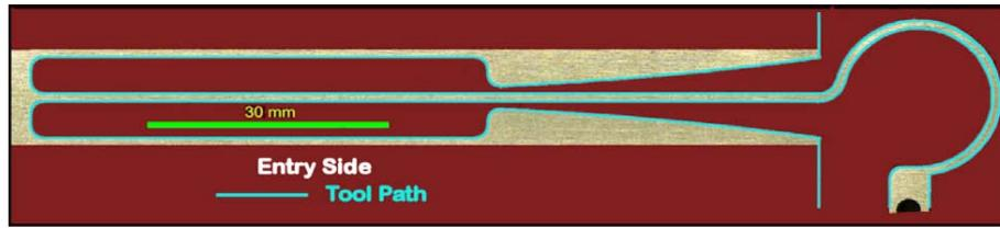
a.  $\mu$ AWJ-cut flexure with tool path
