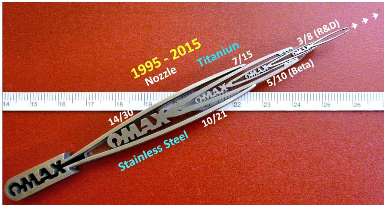
Figure 2: Progress in AWJ meso-micro machining (Liu, 2015)
