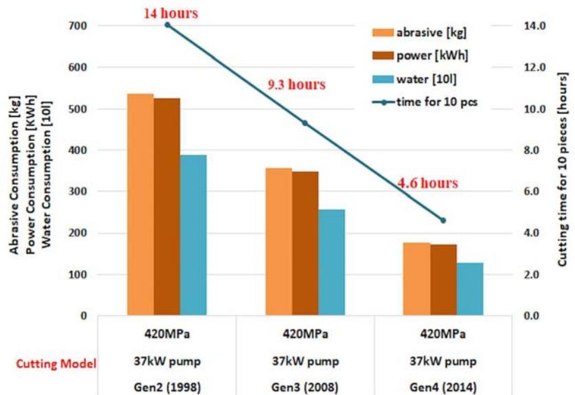
b. Cutting speeds of three cutting models (Henning and Miles, 2016)
