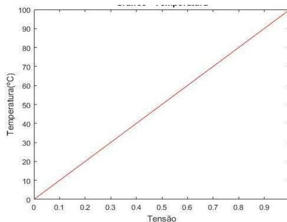
Figure 3: Temperature vs. sensor output voltage graph (LM35)
