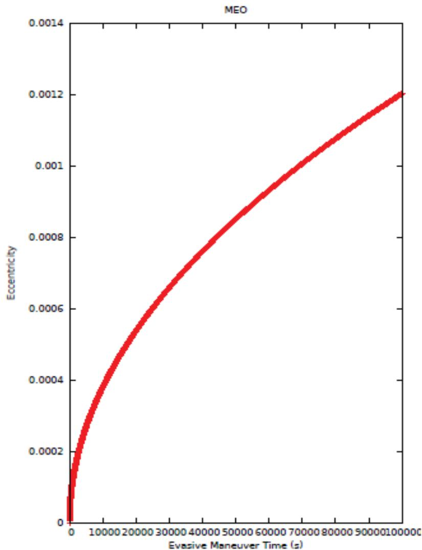
Figure 11A: Variation in the satellite eccentricity by the time. The satellite is in MEO, the gas exhaust velocity is 2.5 km/s, the mass factor of 10, the power factor of the engine is 10–10 1/s.
