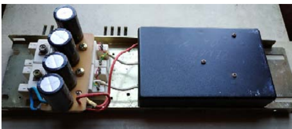
Figure 11: IR2110 circuit assembled with IGBT's.
