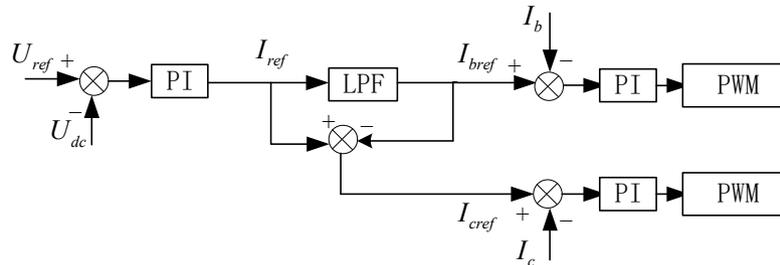
Fig. 5: Voltage and current double closed-loop coordination control strategy
