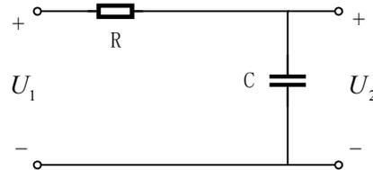
Fig. 4: Circuit diagram of one-order low pass filter
