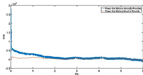
Fig. 7: Actual and reference power of battery
