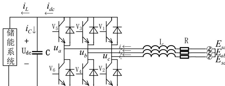
Fig. 3: Equivalent circuit model energy storage converter
