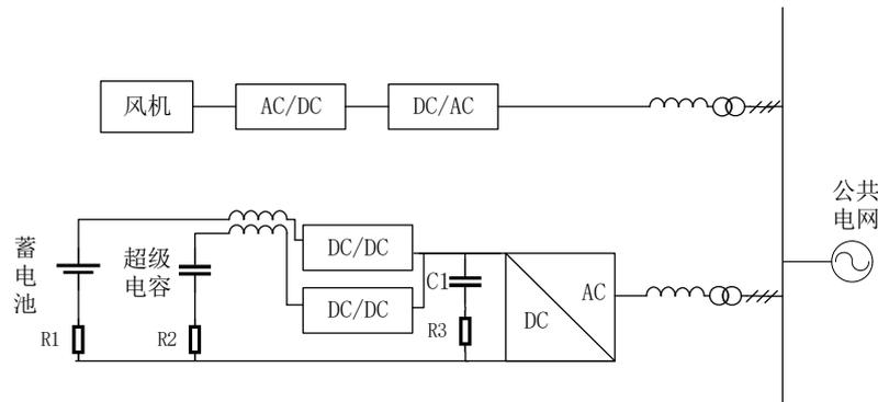
Fig. 1: Structure of wind turbine-energy storage system
