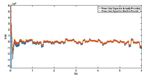
Fig. 8: Actual and reference power of capacitor
