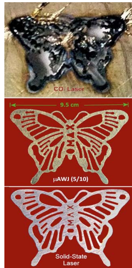
Figure 5: Miniature butterflies machined with lasers and \mu\text{AWJ} (Liu, 2017c, 2019a)
