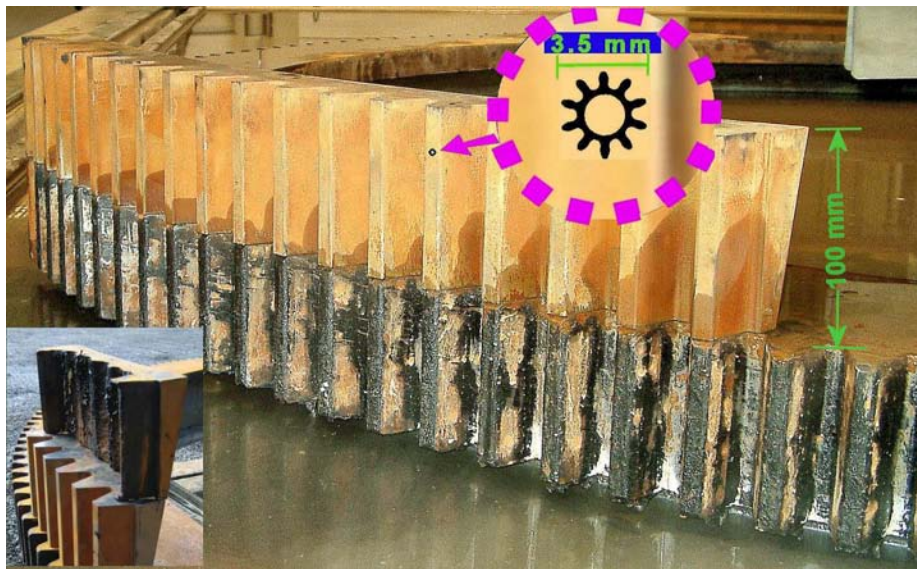
Figure 4: Macro to micro machining with AWJ (Liu, 2017a)
