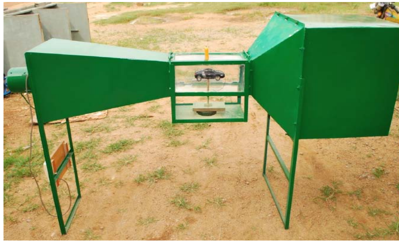
Figure 8: Close Test Section Wind Tunnel, source: [53]
