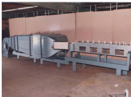
Figure 9: Blower WT, Image source: https://www.aerolab.com/products/blow-down-wind-tunnels/
