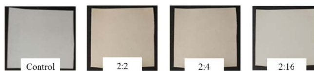
Figure 2: UH050 control and modified membranes with concentrations of DA/PVP of 2:2; 2:4; 2:16 mg mL -1 and deposition time of 2h.
